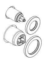
Install both handles by tightening grub screws with provided allen key and inserting grub screw covers.
