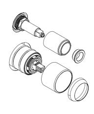
(3) Slide backplate over both sleeves ensuring not to scratch.
